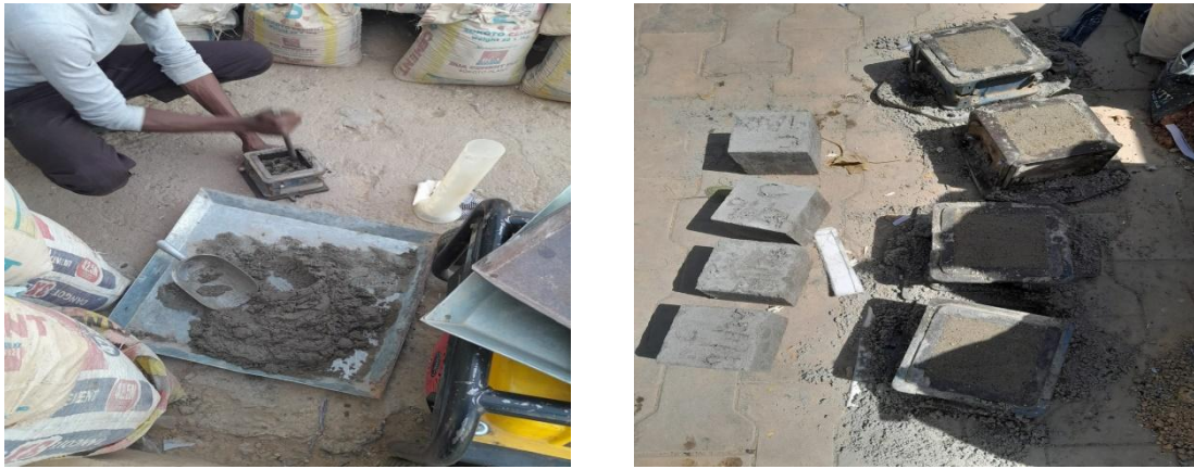
Figure 5. Preparation of companion 100 mm cubes
