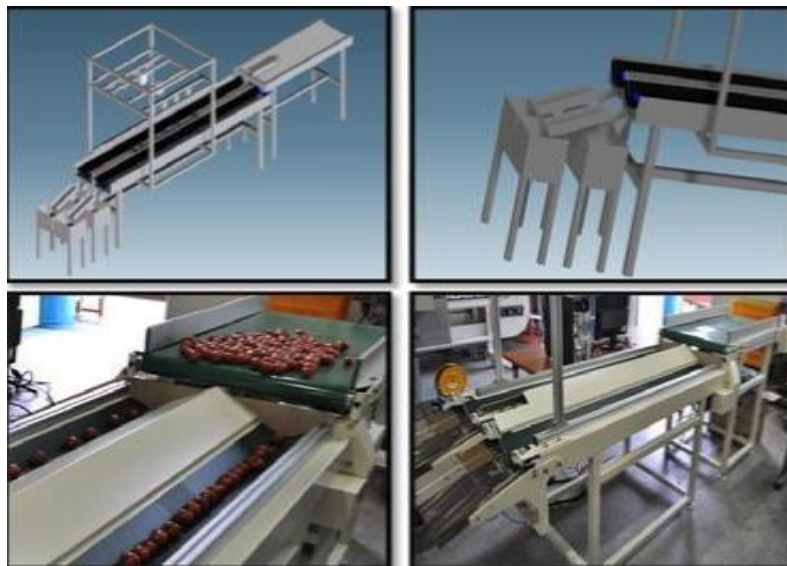
Plate 4: Schematics and photo of the prototype of the colour sorting machine
