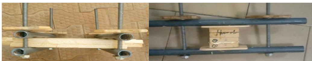
Figure 2: Improvised clamping device for pressure application
