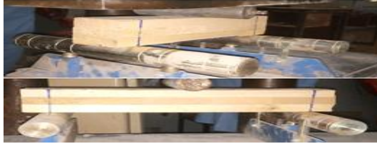
Figure 6: Experimental set-up for three-point short span bending test
