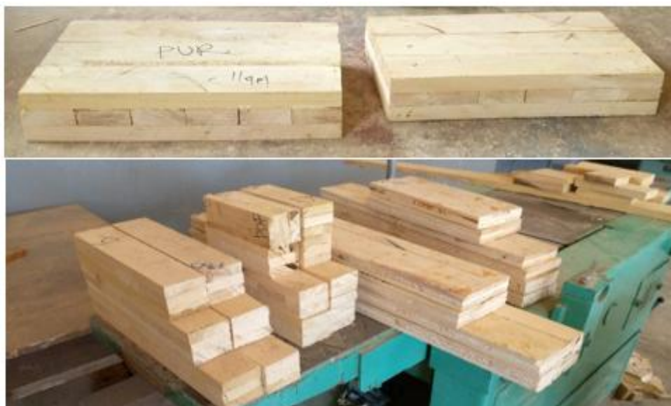
Figure 5: The 3-layer CLT panels and the extracted specimens
